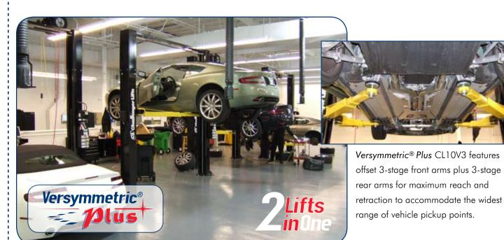
The Versymmetric® Plus CL10V3 provides open door clearance for lifting asymmetrically or symmetrically, and accommodates vehicles with short and long wheelbases, designated outside pickup points, uni-body and wide body imports.
