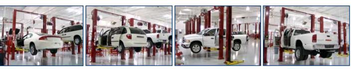
Versymmetric® and Versymmetric® Plus Lifts provide open door clearance for lifting asymmetrically (Dodge Intrepid and Caravan) or symmetrically (Dodge Ram 1500 and 3500 Dually).
